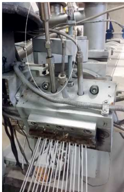
Picture 1: ColVisTec Probe in a Twin Screw Extruder (see marking) – Image Courtesy of KraussMaffei Extrusion GmbH, Germany
