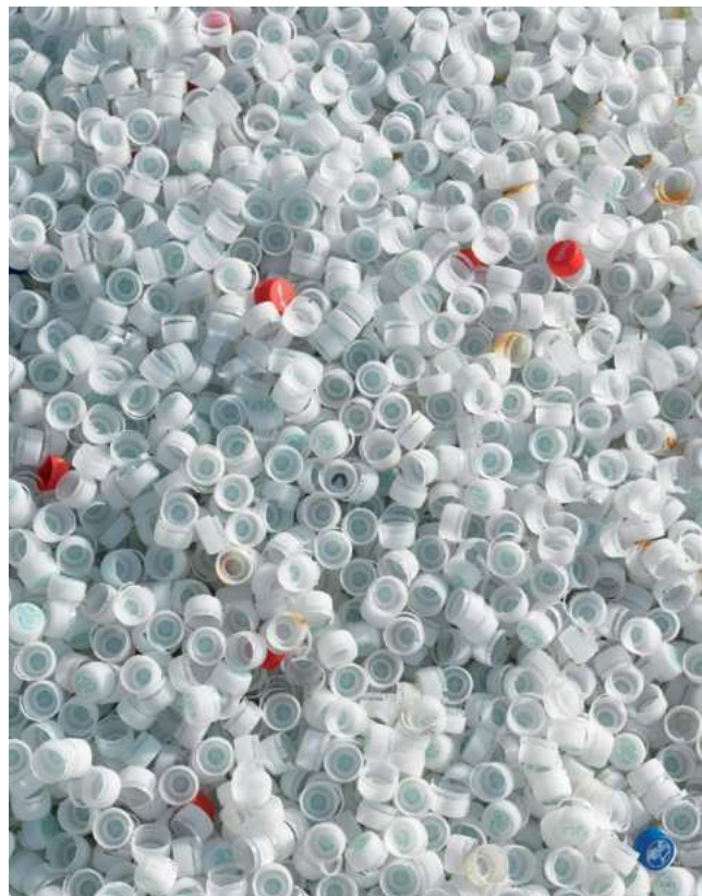
The Starlinger recoSTAR super-cleaning technology turns PP beverage bottle caps into high-quality rPP that can be used at levels up to 100 % in food-contact packaging (© Starlinger)
